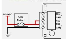
Example: DOTL alarm, Red LED and Sounder activated together from one output.
